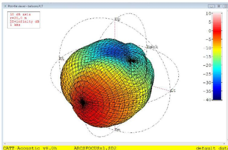
e) Click **All** to display the acoustic field (balloon) produced by the array at each octave-band from 125 Hz to 16 kHz (toggle between screens).
